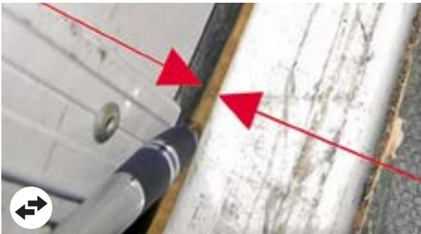
Deformations in the rails not beyond economic repair, closure not possible or not sand-proof
