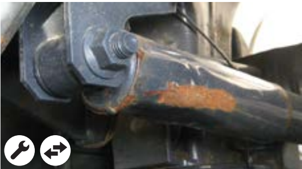
Serious scratches as deep as the primer
