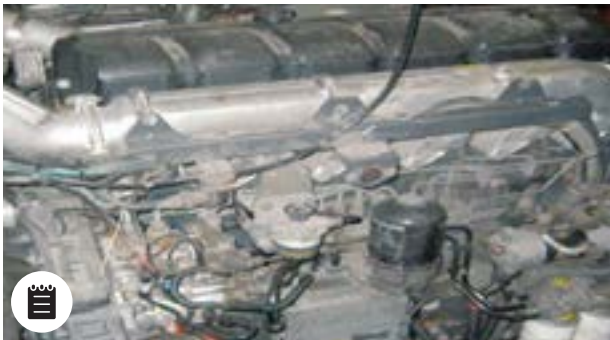
Light traces of oil (no dripping)
