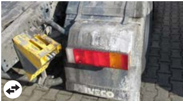
Deep discolouring due to chemical elements
