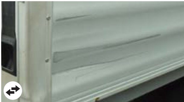
Deformations in the rails not beyond economic repair, closure not possible or not sand-proof
